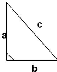
Have a look at the triangle above. This kind of triangle is called a right-angled triangle because the angle on the inside of sides **a** & **b** is  $90^\circ$ . Now, imagine you know the length of side **a** and the length of side **b** but you don't know the length of side **c**. Is it possible to calculate the length of side **c** without measuring it?
